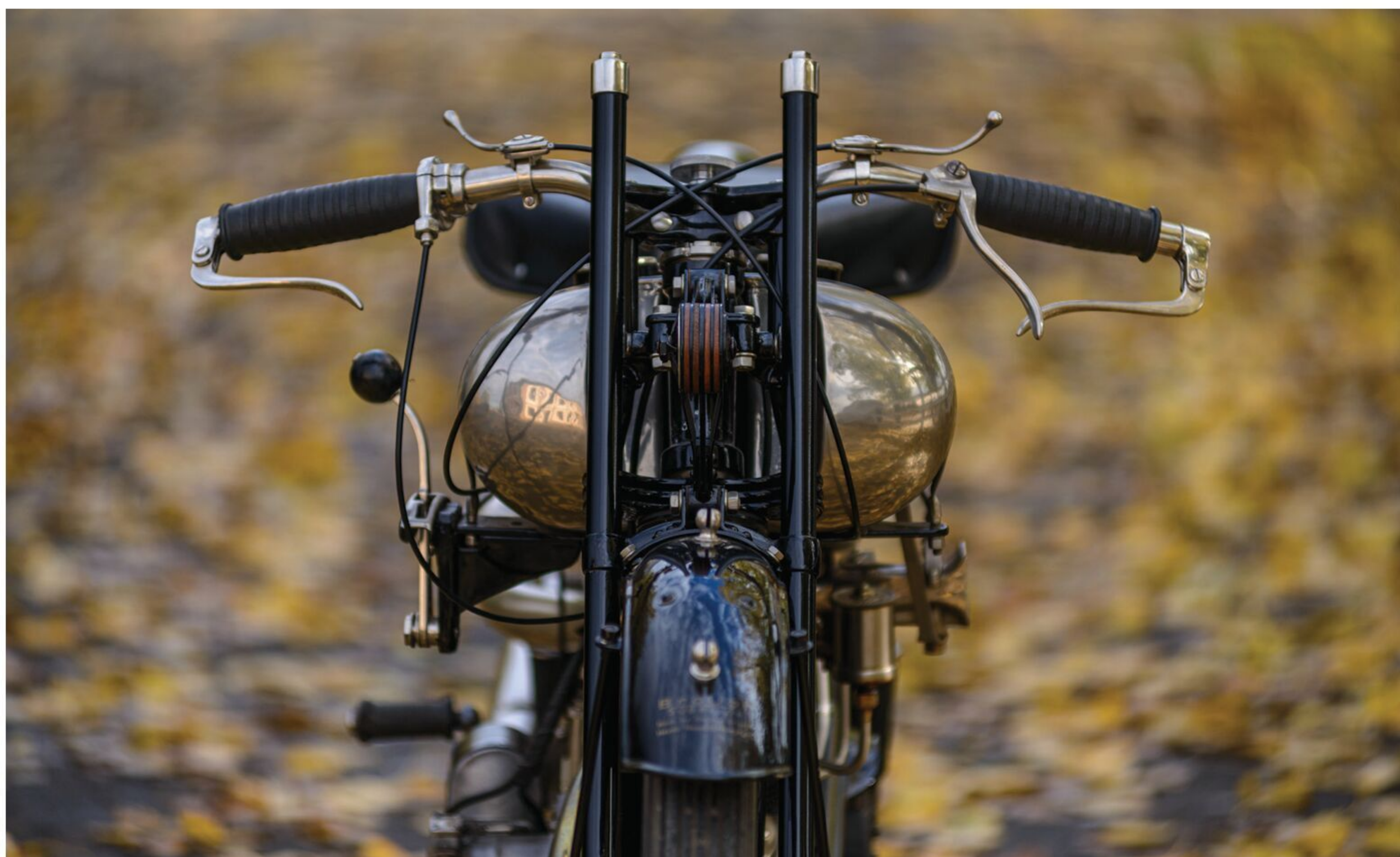
Brough' has patented his modified Harley-styled Castle front forks together with Harold Karlake.
