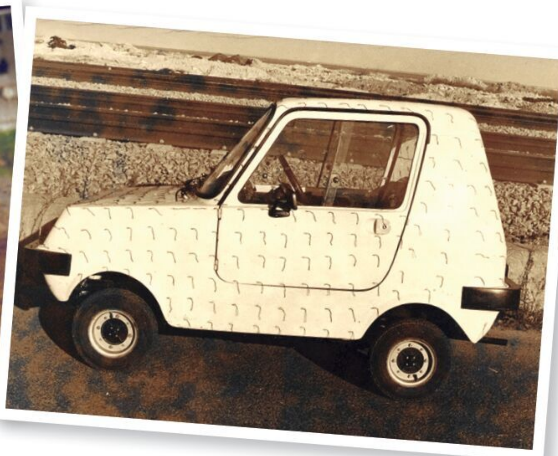
Aerodynamics were tested by gluing yarn strips to the body.
