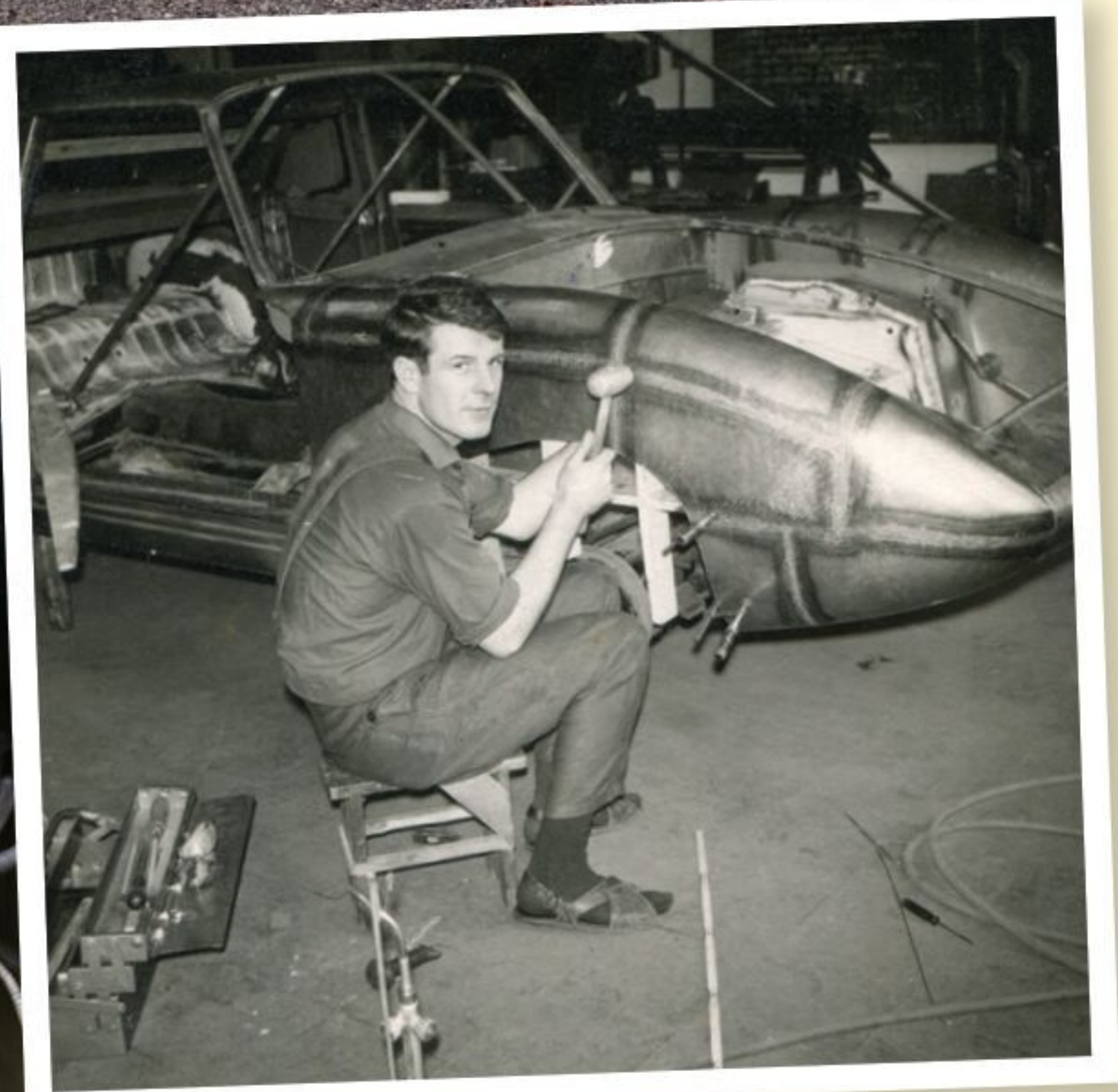
Car was built in sections then welded together.
