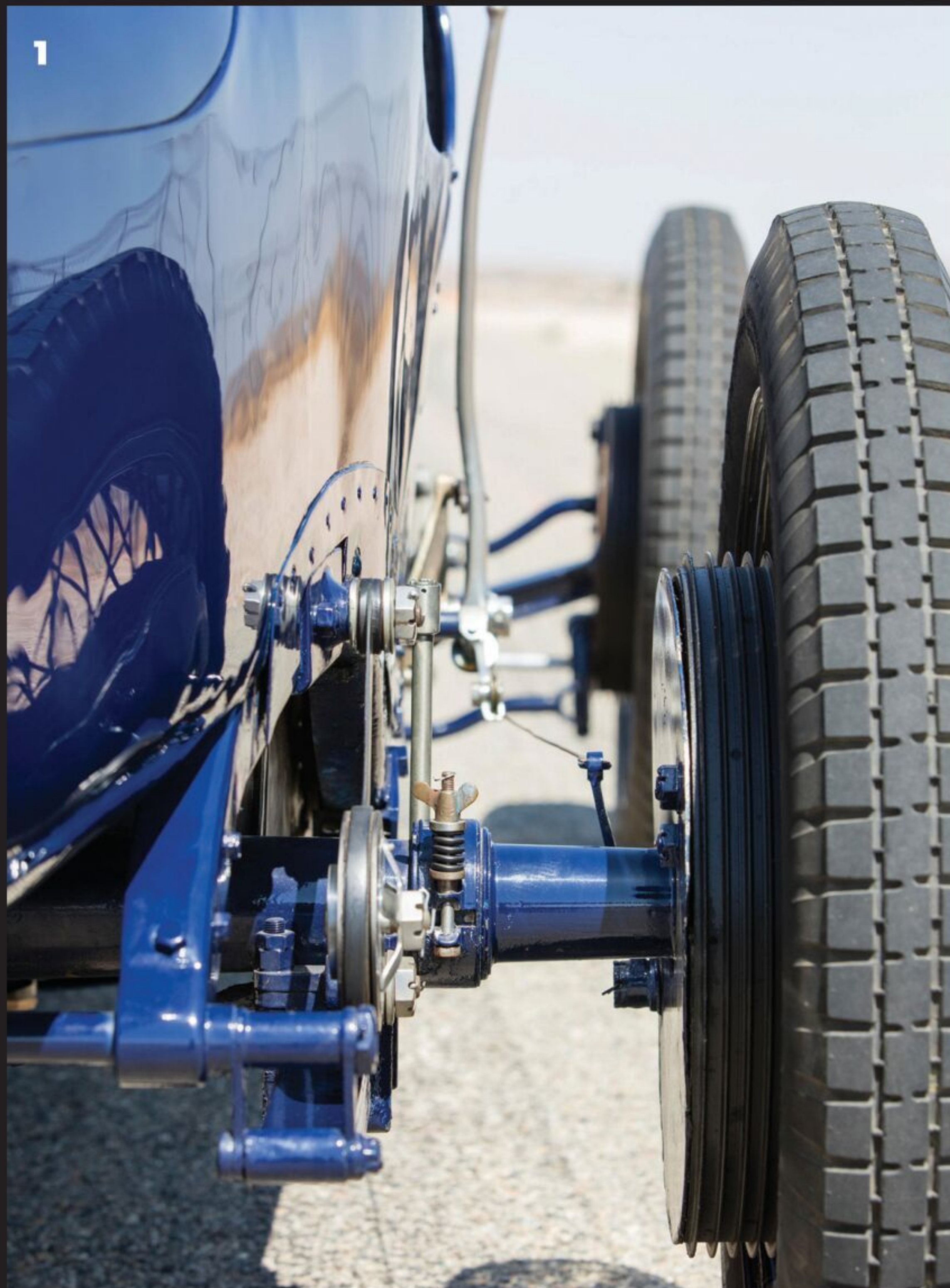
1: Detail of the suspension on L45-01. Note the brakes on front and rear wheels.
