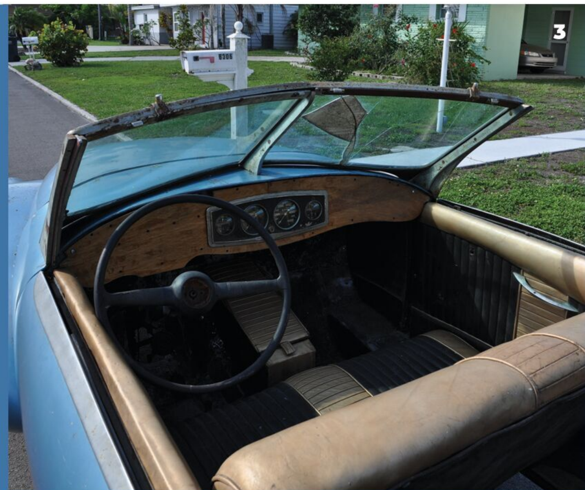
3: The interior of the Kurtis was leather throughout and late 1940s Stewart-Warner instrumentation – all still in place when the car was found.
