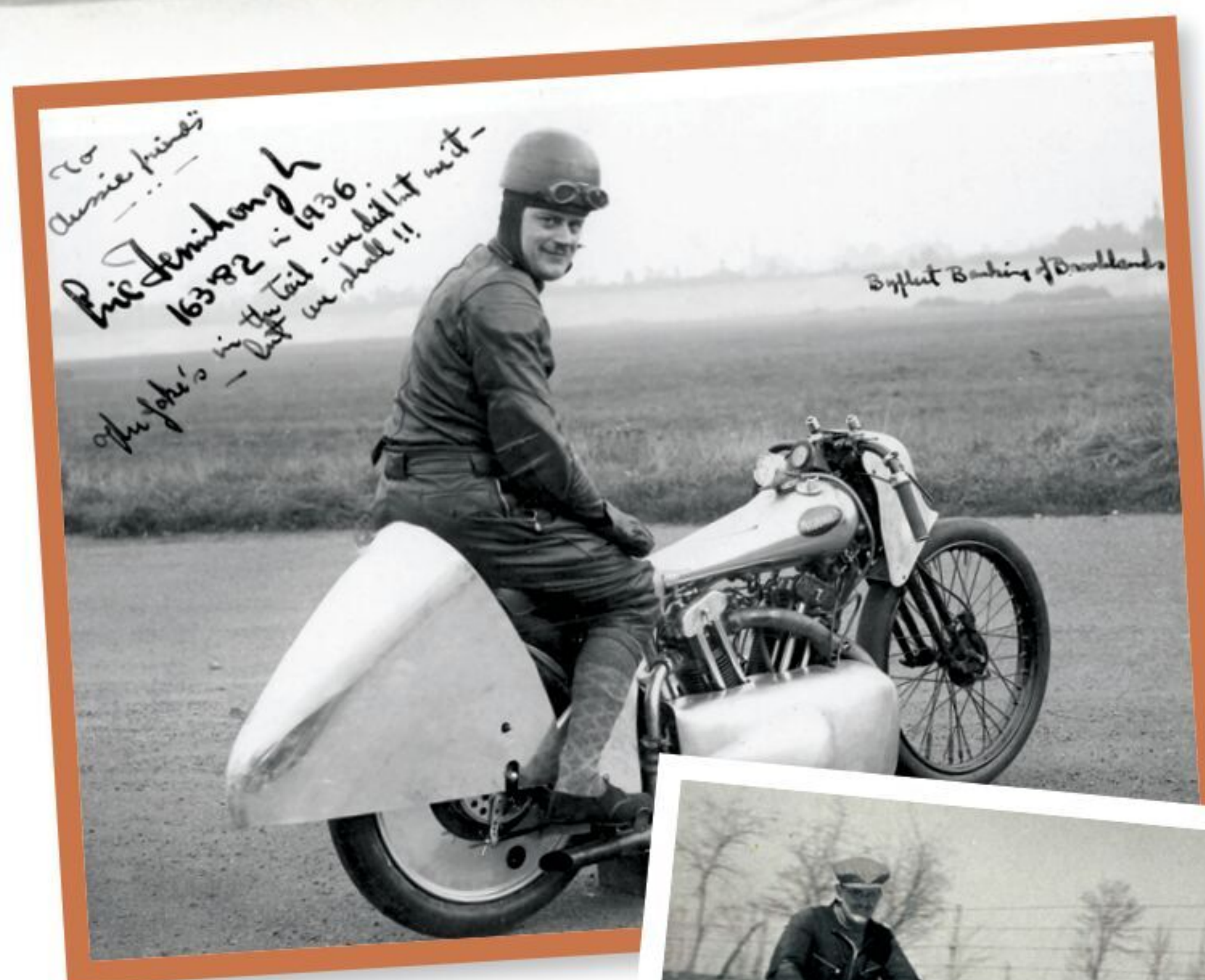
This photo was sent by Eric to a young fan in Australia in 1937. The tail fairing was abandoned after testing at Brooklands and replaced with a more substantial unit.
